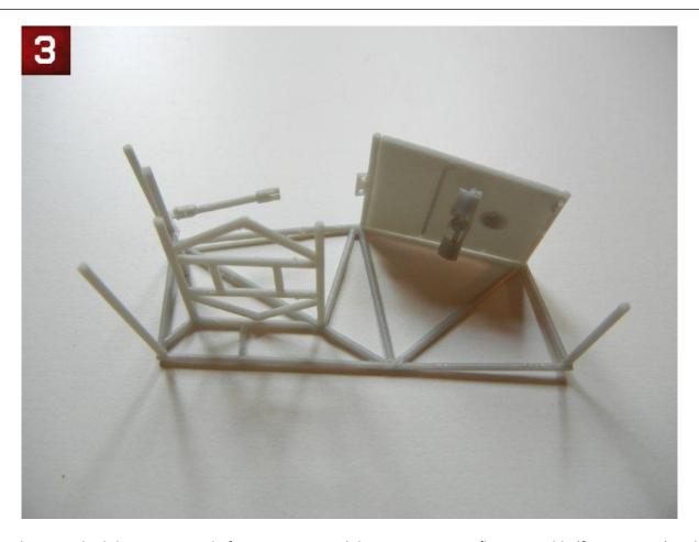
• I then attached the opposite side framing piece, and the MG ammo tray/box assembly (from step 10) and made sure everything was aligned. I also attached the control column, fitting it into the other end of the bracket/rod that was already attached to the bell crank (see photo 4).
