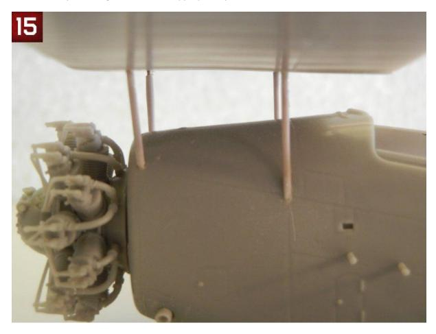
• Attach the outer upper wings to the wing center section, setting the dihedral at 11mm at the outer tip. Again, see the article "Making Templates" in the "Tips and Reviews" section of the Silver Wings website (www.silverwings.pl) for tips setting the correct dihedral. When dry, my wings had slight gaps on the underside, which were filled by the superglue used to join them (see photo 16).
