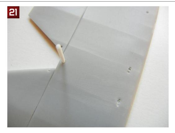
• Drill out the support brace holes in the bottom of the tailplane and test fit the tailplane to the fuselage. Using the support brace, determine the appropriate forward fuselage attachment position, and mark and drill the attachment hole (there is no pre-sunk hole for this part) see **photo 22**.
