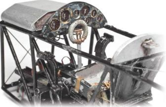
Acetate dial faces were sandwiched between an etched control panel face and a plastic card backing. The instrumentation is rather impressively done, each dial being clearly legible..
