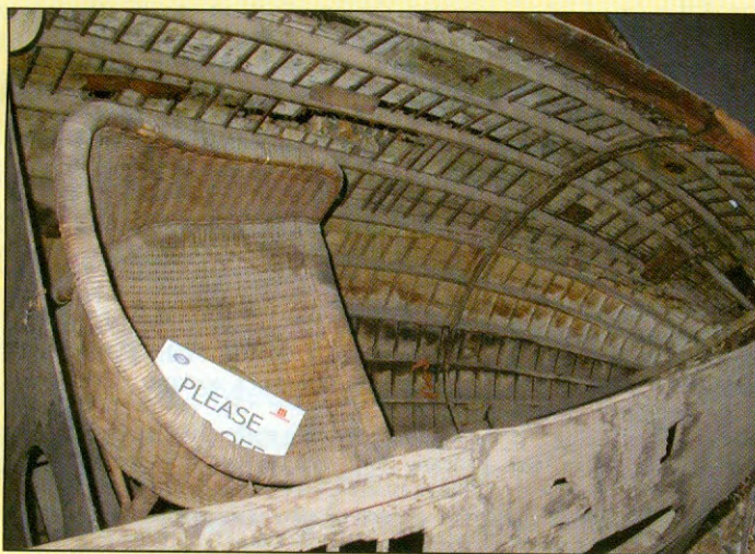
Judging from a few remnants of paint shown on this hull section, the interior colour of the aircraft was most likely to be white.
